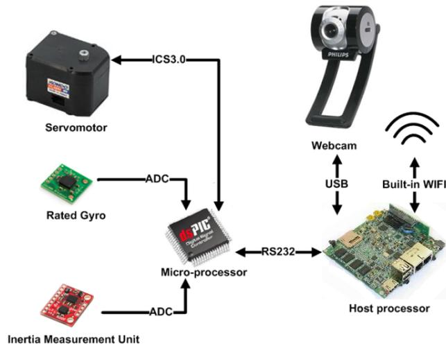
**Fig. 2.** Robo-Erectus Architecture
